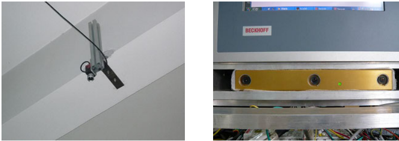
Fig. 1. Ceiling cameras and trinocular vision
